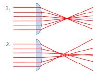
Figure 3: Diagram 1 shows the focal point of a perfect lens, while diagram 2 shows an imperfect lens displaying spherical aberration.
