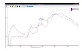
Figure 1: Sensitivity in the UV is enhanced for concave holographic spectrometers. Comparison of BLACK-Comet sensitivity (blue line) compared to plane grating spectrometer (red line).
